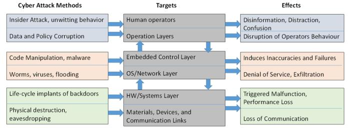
Fig. 1. Potential cyber-attack methods, targets and effects
